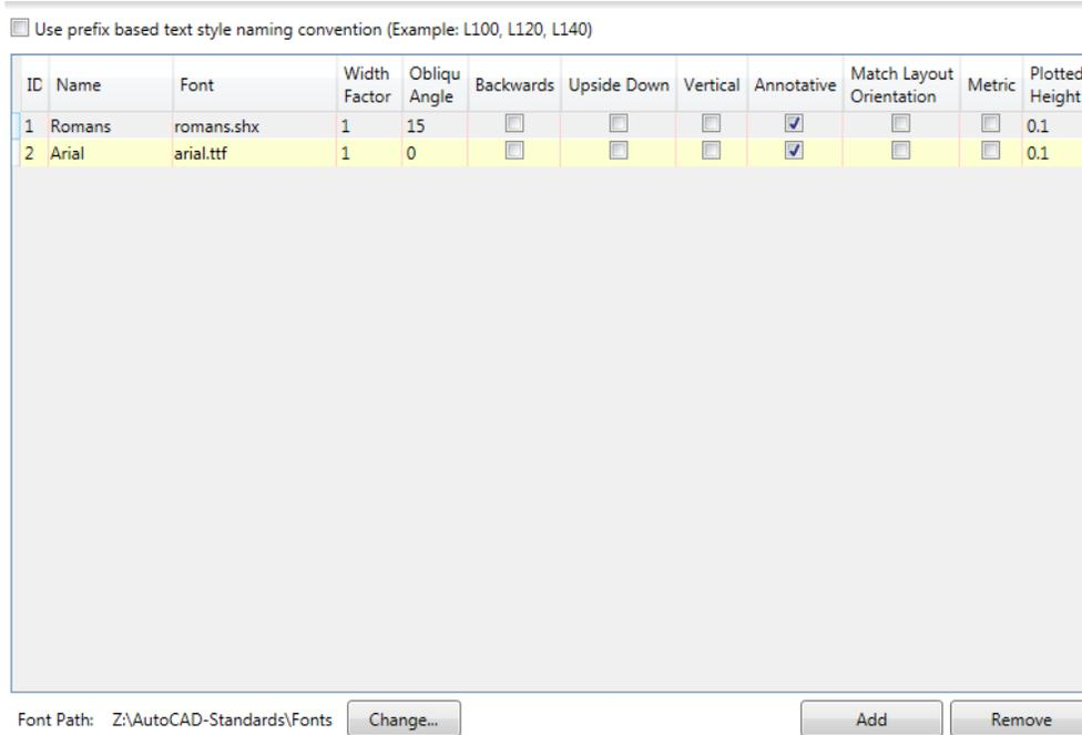
Text styles can be created based on two different naming conventions. One based on a single name for each text style and the second based on a prefix name and text height.
