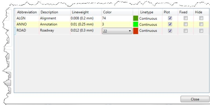
Once the component is entered, the layer property default should be added. This sets the default for any layer created from the rightmost layer component other than ^, none/null, which is ignored. If setting up a standard for the first time, it is highly recommended that you use this feature to help when creating the layers.
