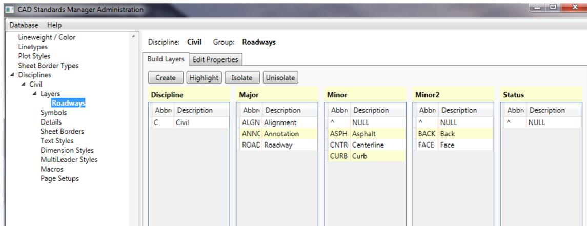
This is the selection in the first pass. After selecting the components below, click **Create**. In this example the layer group was named Road Layers.
