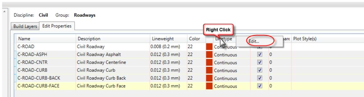
To assign properties to several layers at once highlight the desired layer names. You may use windows selection techniques or click and drag the mouse over the layer names. Once you have selected all the desired layers, right-click the desired column header and choose Edit to modify multiple layers at the same time.
