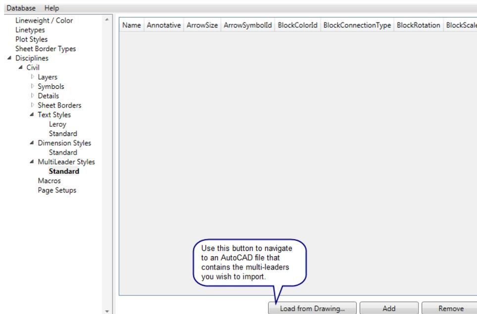
To remove a multileader style from the standards database, simply select the desired row(s) and select the **Remove** button.
