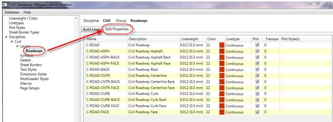
Notice that every possible layer combination from the highlighted components was added together. This interface above allows the administrator to remove layers from this group as well. Therefore, it is often more efficient to add layers to a group multiple times to get the desired effect.
