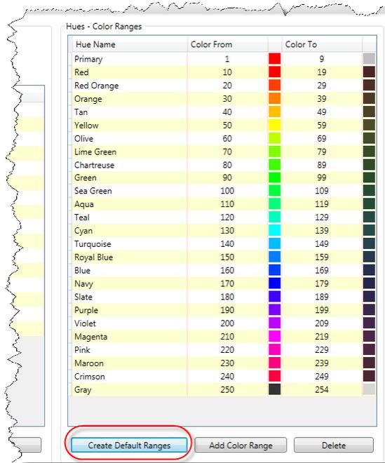
In the above example the **Cyan** hue contains the colors 130 through 139. The lineweight .35mm corresponds to color 131 in that hue range. Assigning the cyan hue range to the "storm drain" layer group will automatically assign the color 131 to any layer in that group with lineweight .024".
