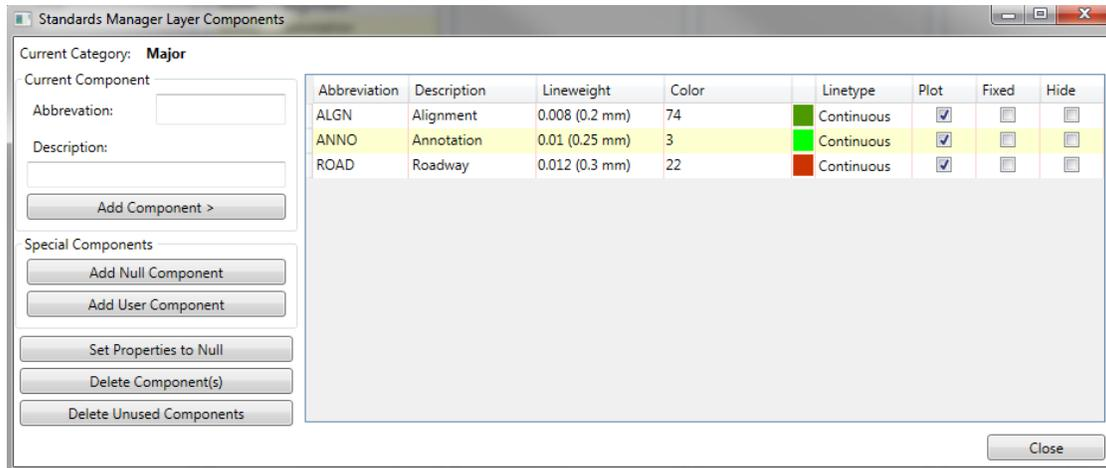
Enter an abbreviation in the field. This will be the component displayed as part of the layer name. Hit <tab> to move to the description field and type a description for the abbreviation. Hit <tab> to move to the **Add Component >** button. Hitting <Enter> a second time will add the abbreviation to the component list and return to the abbreviation
