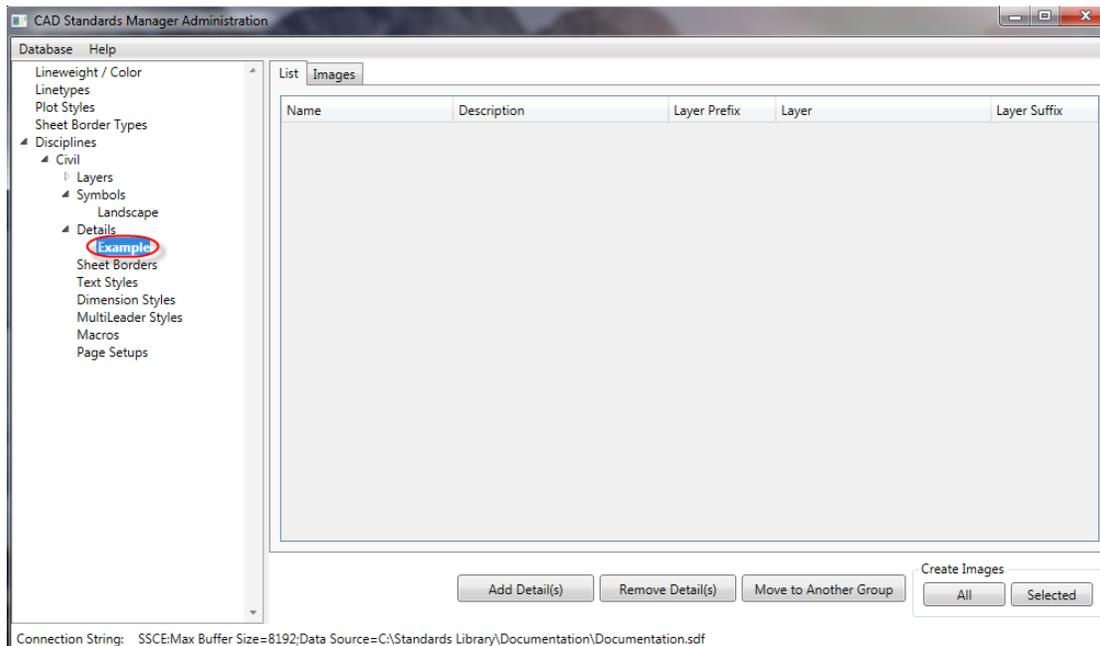
Once you have imported your details you can add a description, an insertion layer and layer prefixes/suffixes. It is important to add a description for the end user as they can query the database to locate the correct detail, this will make it faster.
